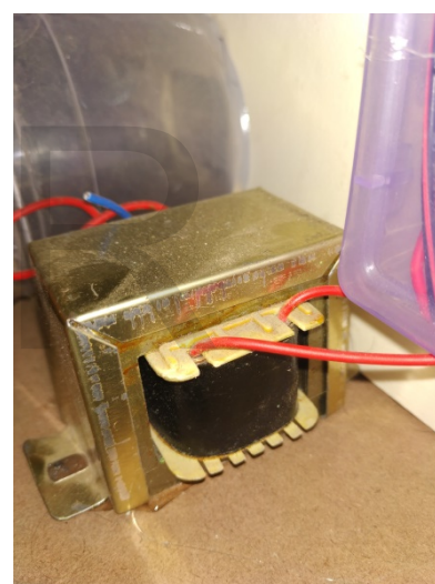
Fig8: Step down transformer
