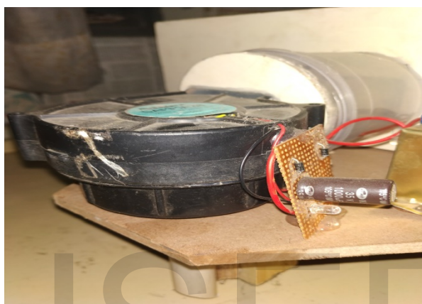
Fig4: Suction fan generating vacuum
